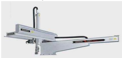
BRR Series is applicable to all types of horizontal injection machine ranges of 100~650T for take-out products and sprues. Vertical arm is telescopic stage. Full AC servo motor driven on each axis. Products take-out at super high-speed (0.8sec.) and dry cycle time within 5 seconds, applicable to take-out products with short forming cycle or complex automatic. Also with the function of mold labeling and mold inserting.
